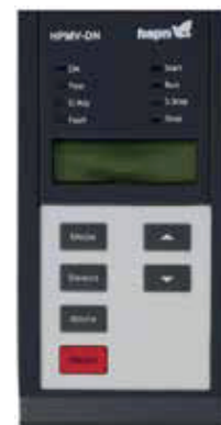
Fig 11 HPMV-DN control panel
